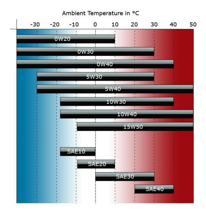
The chart above illustrates a rough guide to ambient temperatures vs oil viscosity performance in both Multi-grade (top half) and Mono-grade (lower half) oils. So you can see that multigrade oils have a much broader spectrum of use.
